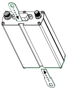
4. Attach the MultiModem with two screws to the mounting surface at the desired location on the equipment.
